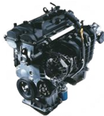
1.2L Kappa Dual VTVT Petrol Engine
