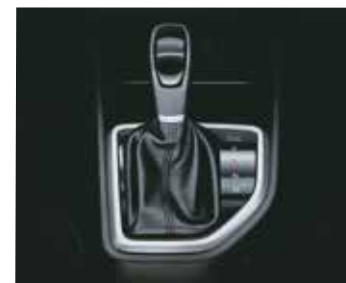
6-speed Automatic Transmission in Petrol & Diesel Variants
